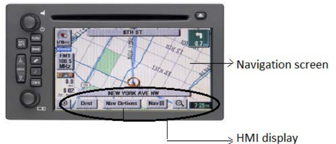
Fig.6: Combination of HMI display and Navigation
