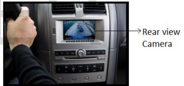
Fig.5: Example showing a Back up Camera which uses frame buffer 1
